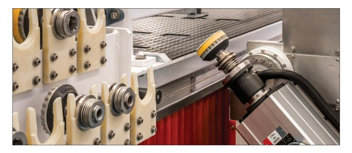
The Edgemaster GEN2 is fully automated and comes equipped with an 8 position Automatic Tool Changer, allowing the machine to work continuously and tirelessly without interruption, improving efficiency and accuracy to the completion of work.
